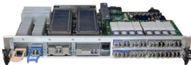
100G/200G Transponder/Muxponder is a full slot, double height card, supporting 10G/25G/100G Ethernet clients with PTP capability
