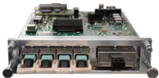
400G Muxponder (4 x 100G clients, 1 x 400G line) is half slot, double height card combining 100GbE and OTU-4 into 400G line
